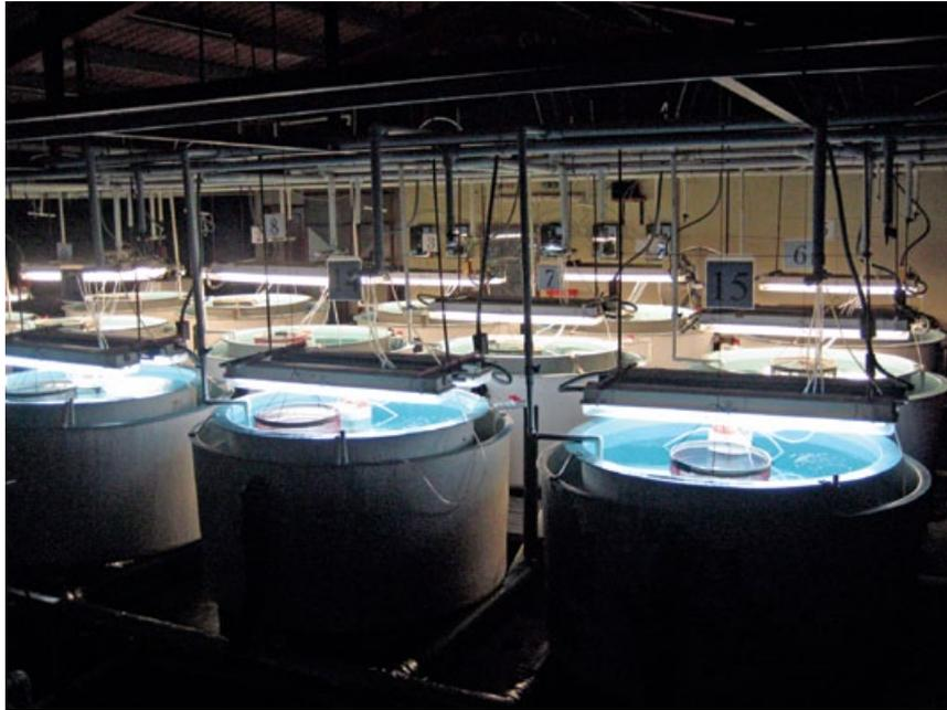
Figure 2. The multiple experimental tanks with nested egg incubators used in experiment 1 and experiment 2 of the pilot study.
