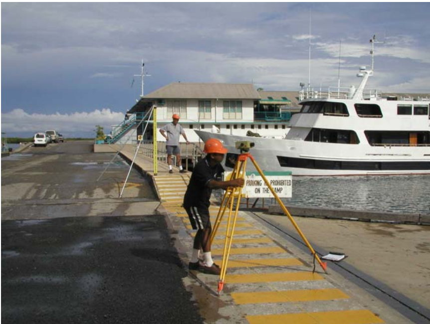
Andrick and Brian carrying out the Precise Differential Leveling at the Kings Wharf in Lautoka.
