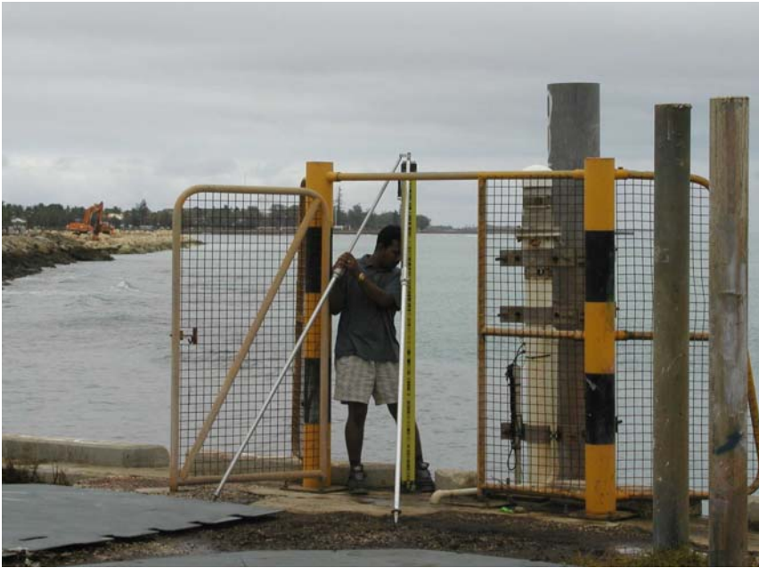
Andrick setting up the Invar bar coded starve on the benchmark at the NTF Tide Gauge stationed at Queen Salote Wharf in Nuku'alofa, Tonga.
