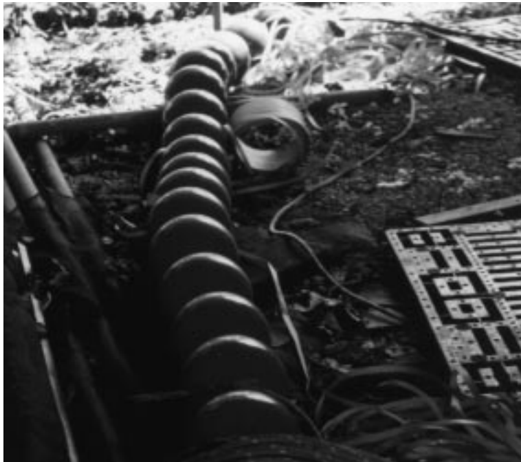
Figure 4: Pressure floats strung together to form the buoy of a FAD
