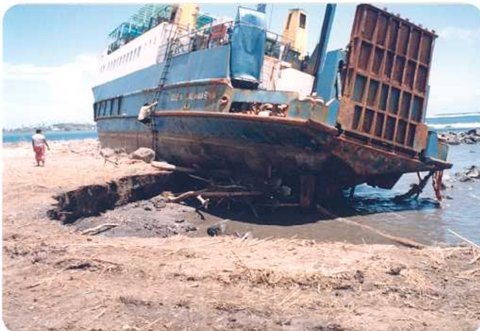
Figure 15. The landfill on which the Queen Salamasina was beached has been severely damaged, losing about 20 meters of fill to the strong waves that attacked the inner harbour area of Apia.
