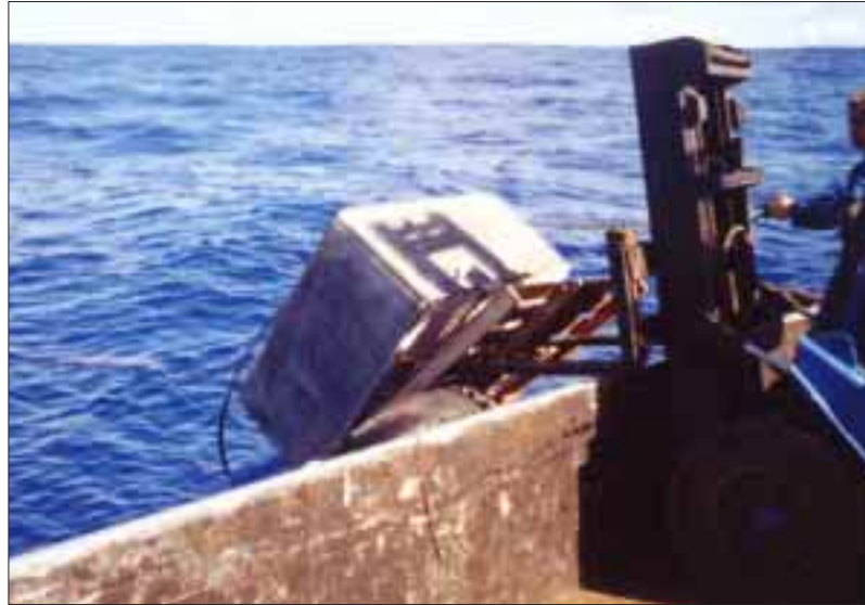
Figure 6: Deploying the FAD anchor block in Aitutaki with a forklift [Photo: Steve Beverly]
