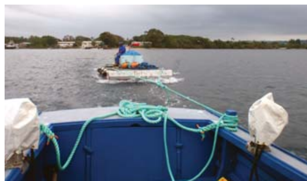
Figure 7. Towing the subsurface FAD on a barge to the deployment site.
