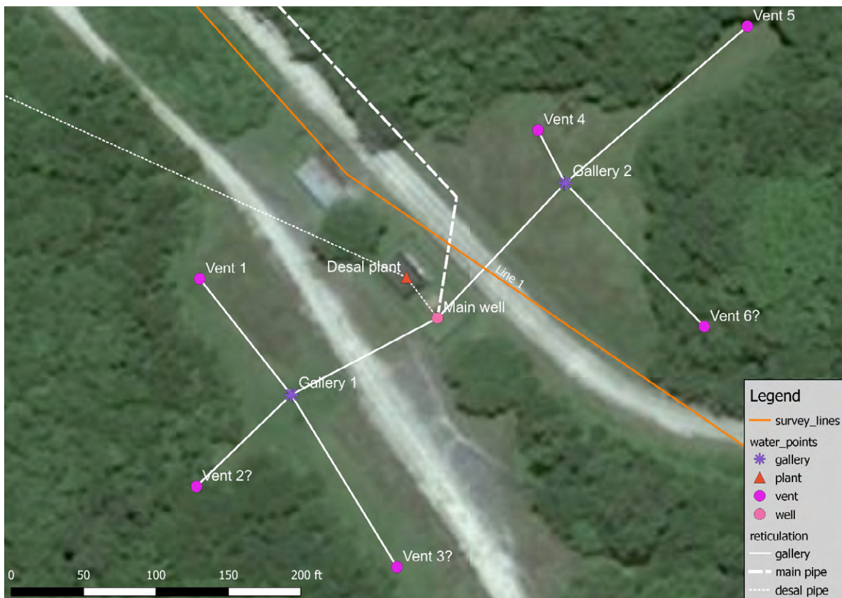
Figure 21. Peleliu's groundwater abstraction and treatment system for public supply. Vent locations 2, 3 and 6 are approximate.
