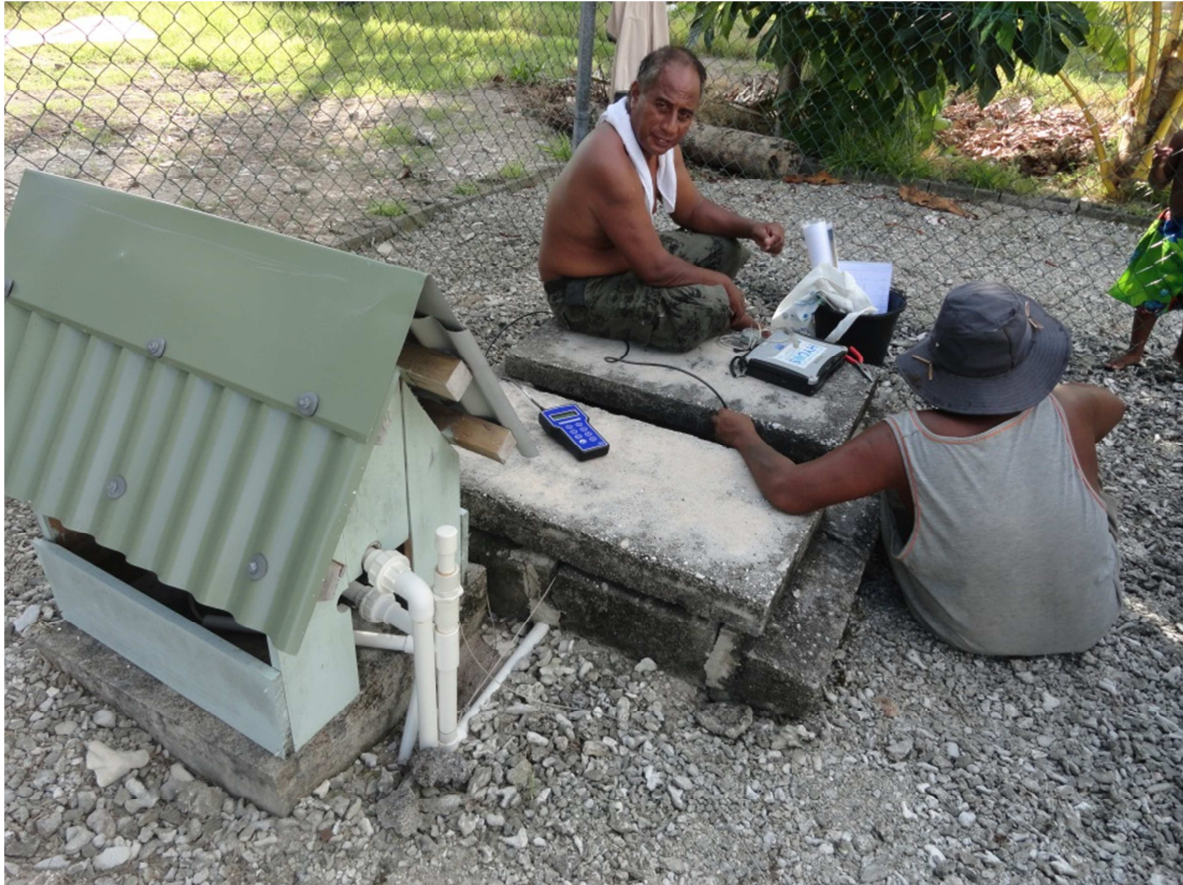
Figure A12-12. Team taking salinity measurements at the village Health Clinic well.
