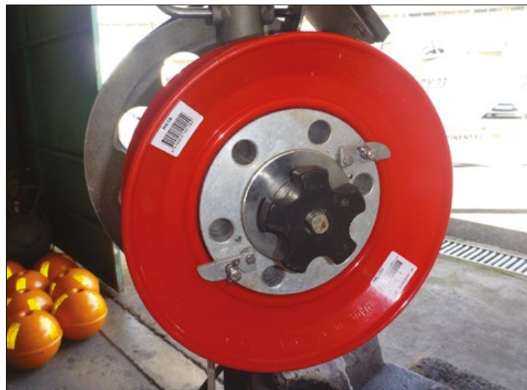
Figure 5. A plastic spool fitted onto the coupling and locked in (image: Mainui Tanetoa).
