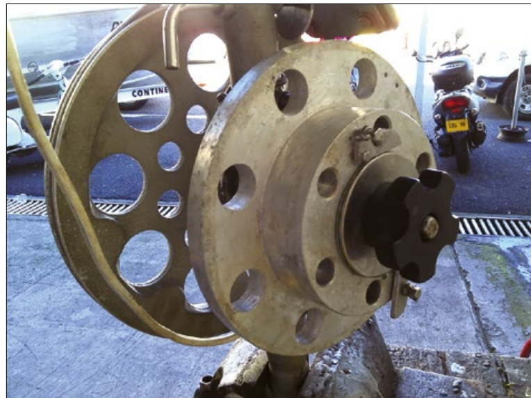
Figure 4. Coupling constructed especially to hold the Alvey hand-cast spools (image: William Sokimi).
