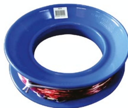
Figure 3. An Alvey hand-cast spool used for holding a single stainless steel mainline (image: William Sokimi).
