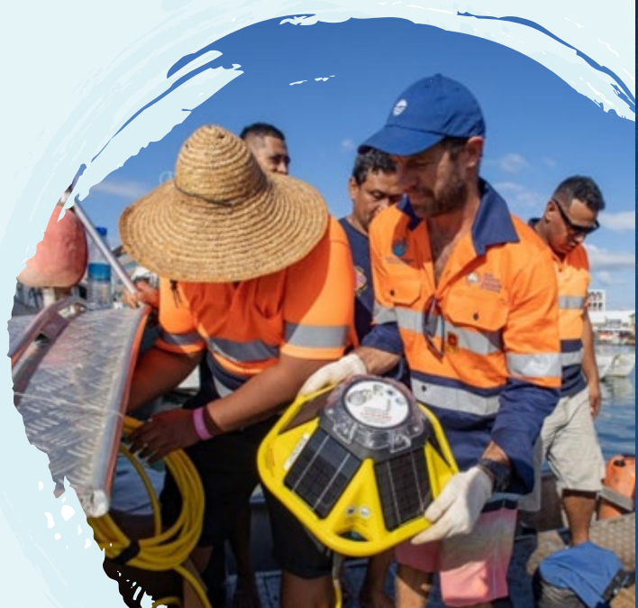
SPC team installing a buoy for wave data collection.
