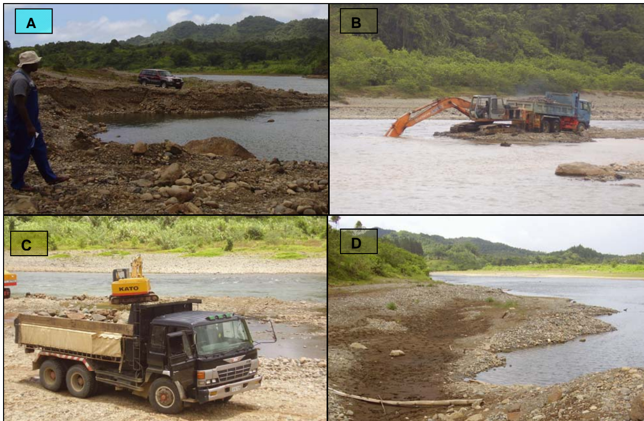
Figure 11. Aggregate extraction and its impacts at Nakavu. A) An extraction pit at the Nakavu extraction site; B) Aggregate extraction from the main river channel in progress. C) Bigger rock boulders extracted from the river channel are taken to the crusher in a dump truck. D) Accumulation of mud in sand bars are becoming more prevalent.
