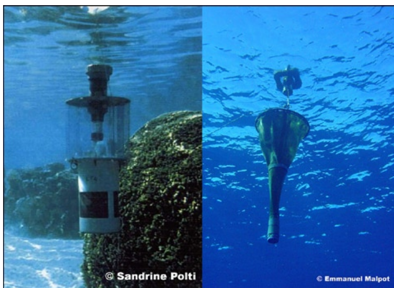
Figure 4. Aquafish Technology light-trap in Moorea lagoon (taken from Polti 2001.) and Ecocean light-trap (CARE system) in sub-surface waters at Rangiroa (taken from Malpot 2005).
