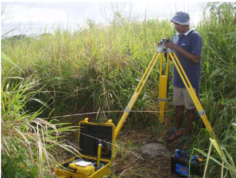
Figure 19. Photograph showing the base station tripod on the Maungapu 41204 benchmark. The Trimble R8 system can be seen in the yellow case in the foreground. Also shown is one of the 12V batteries used to power the system.
