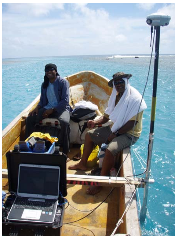
Figure 20. SBES setup on MMR vessel. Note the Trimble R8 GPS on top of the transducer pole (actual transducer is out of sight). The laptop running Hypack 2008 is seated on top of the Echotrac CVM topside unit. The equipment was powered by 12V battery with an AC inverter.
