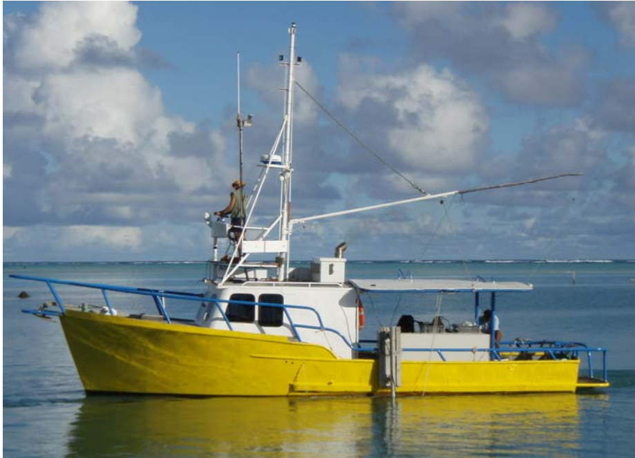
Figure 18. The chartered survey vessel, Orongo. Note the over-the-side pole-mount of the MBES amidship .
