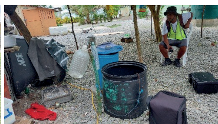
Figure 11. A black 200-L plastic drum used as casing material with the rope attached to the bottle for accessing the groundwater.
