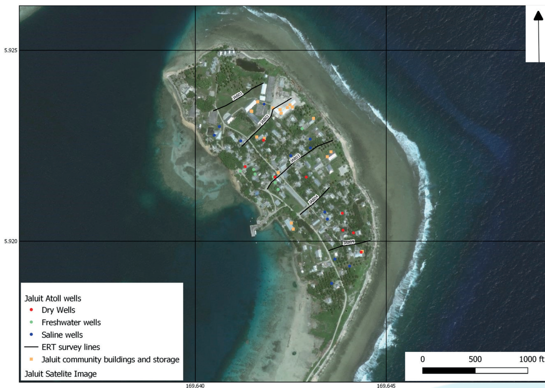
Figure 14. Jabor water resources assessment map showing the location of hand-dug wells, communal buildings and storage tanks, and resistivity survey lines.
