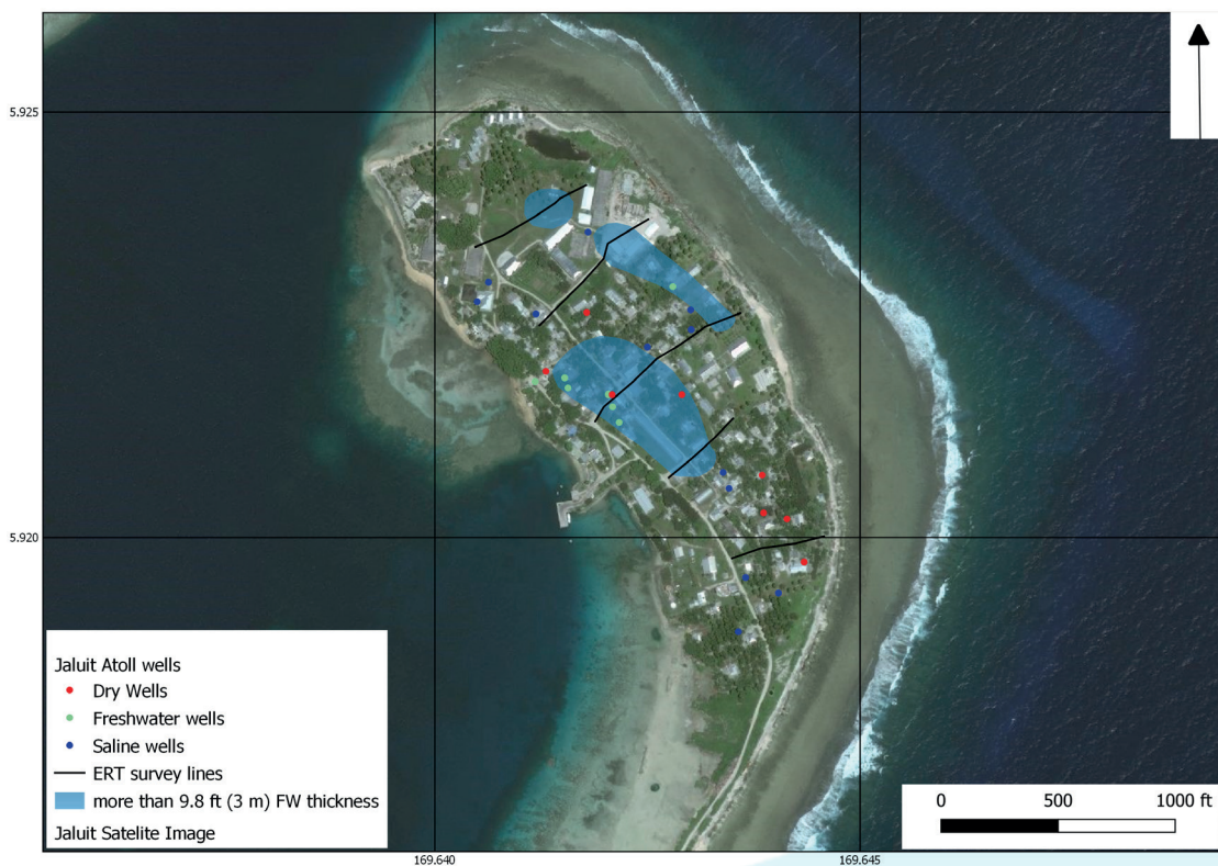
Figure 19. Freshwater lens thickness contours and salinity levels (as EC) in private wells on Jabor islet.
