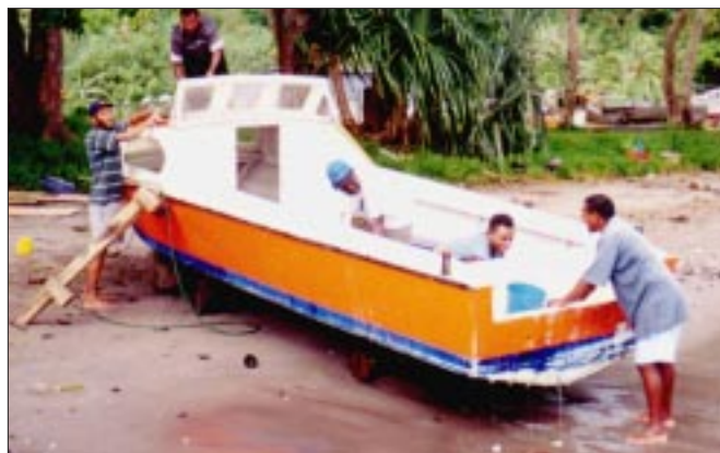
Four boats were pulled ashore on coconut-log rollers... ...and thoroughly cleaned inside and out.
