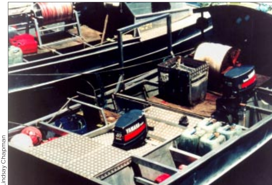
Figure 1: The 9 m class outboard-powered alias
