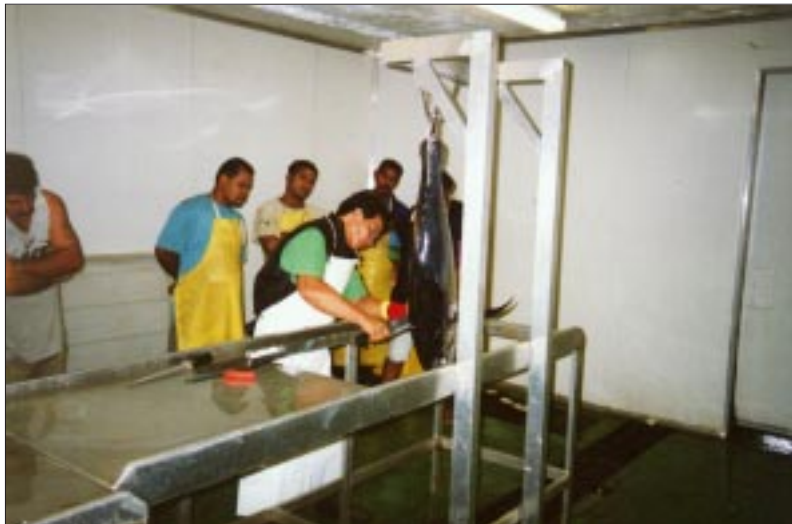
Unique in Tahiti, the fish is hung by the tail for the initial cuts that remove the head and the half-loins from the frame
