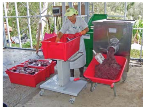
Figure 4. Grinding tuna waste for the production of fish silage (fertiliser) (image: BioAgri-NC).
