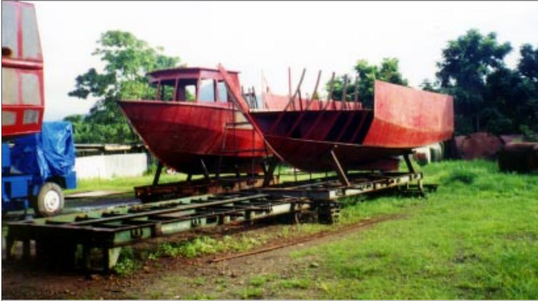
Figure 2: Ten-metre deep-bottom fishing vessels under construction
