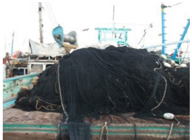
Tuna gillnets are extremely large, and each vessel carries 2.5 to 3.0 tonnes of nylon nets. ©Muhammad Moazzam
