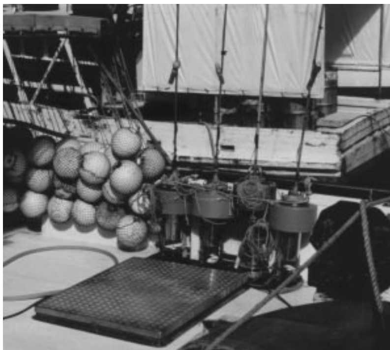
Figure 4: Radio beacons with lights and floats used in longlining operations
