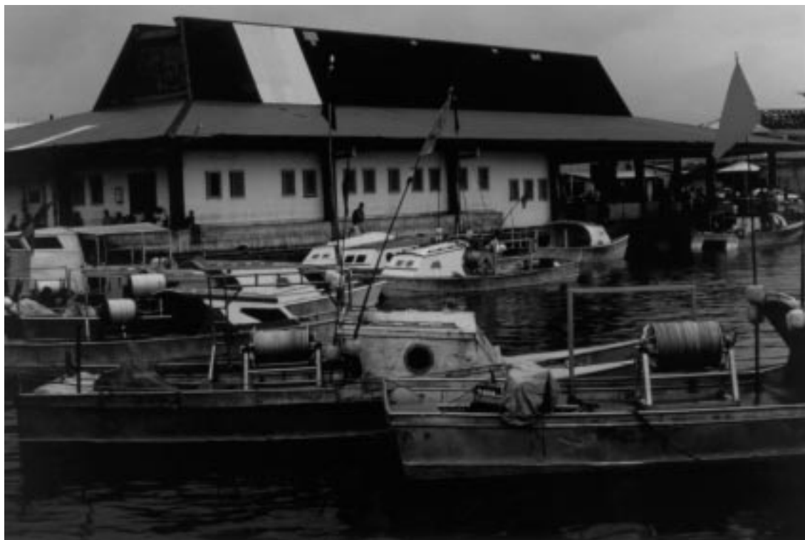
Figure 9: Some alia catamarans rigged with tuna longlining gear in Apia harbour
