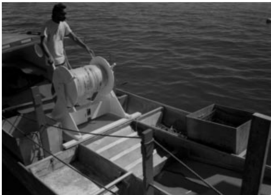
Figure 4: Wooden reel with vertical longlines mounted on an alia catamaran
