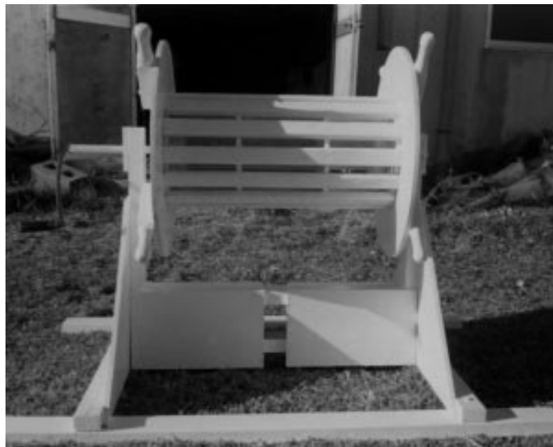
Figure 3: Wooden reel constructed for storing and using vertical longlines
