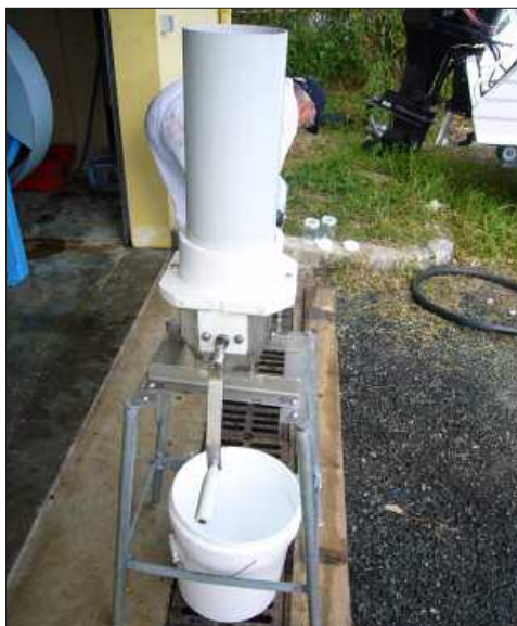
Top. The large fish cutter; typically used in New Zealand's longline fishery in the Southern Pacific Ocean. This model was purchased second-hand and was reconditioned prior to its shipment to Lifou. The inside view of the cutter shows the steel shaft that is made of a series of hammers, which pre-breaks fish waste on a corresponding series of anvils.
