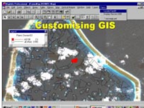
The picture shows the display of a farm search written by the workshop participants in MapBasic. The operator is requested to type the farm ID and the program displays the corresponding farm in red, centres the farm and zooms in.
