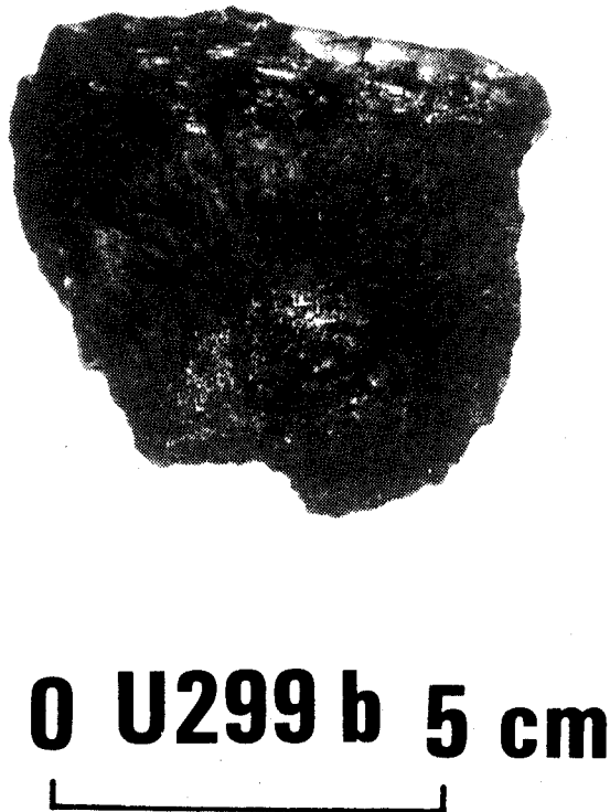
Figure 6. Stn U299b manganese crust fragment; cross-sectional view, upper crust surface at top (eastern margin of Manihiki Plateau, depth 4469-4464 m).
