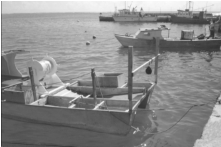
Figure 3: Wooden vertical longline reel mounted on the fisheries alia
