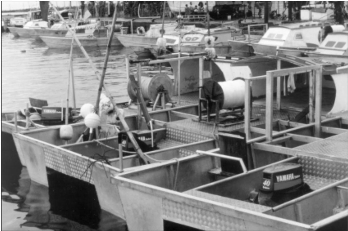
Figure 5: Some alia catamarans with tuna longline gear at anchor in Apia Harbour
