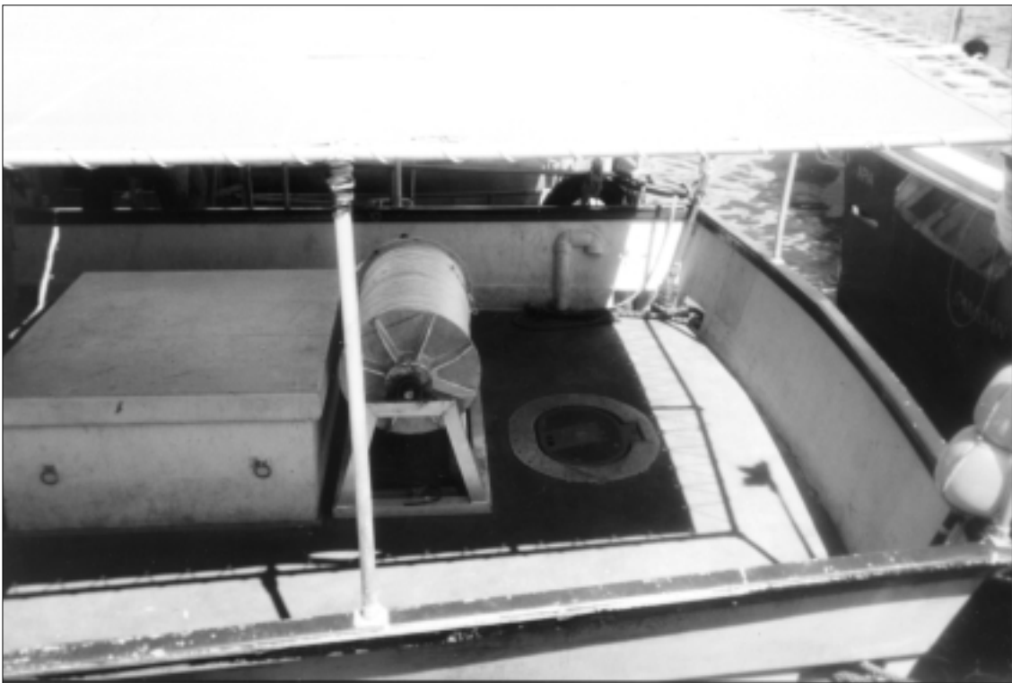
Figure 8: Hydraulic longline reel mounted behind fish hold hatch
