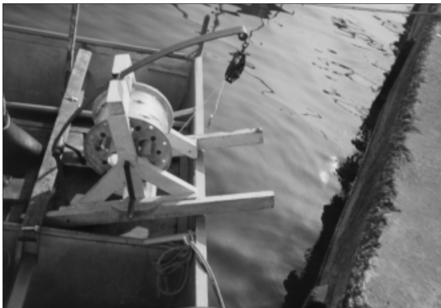
Figure 4: A vertical longline reel design developed by a local alia fisherman
