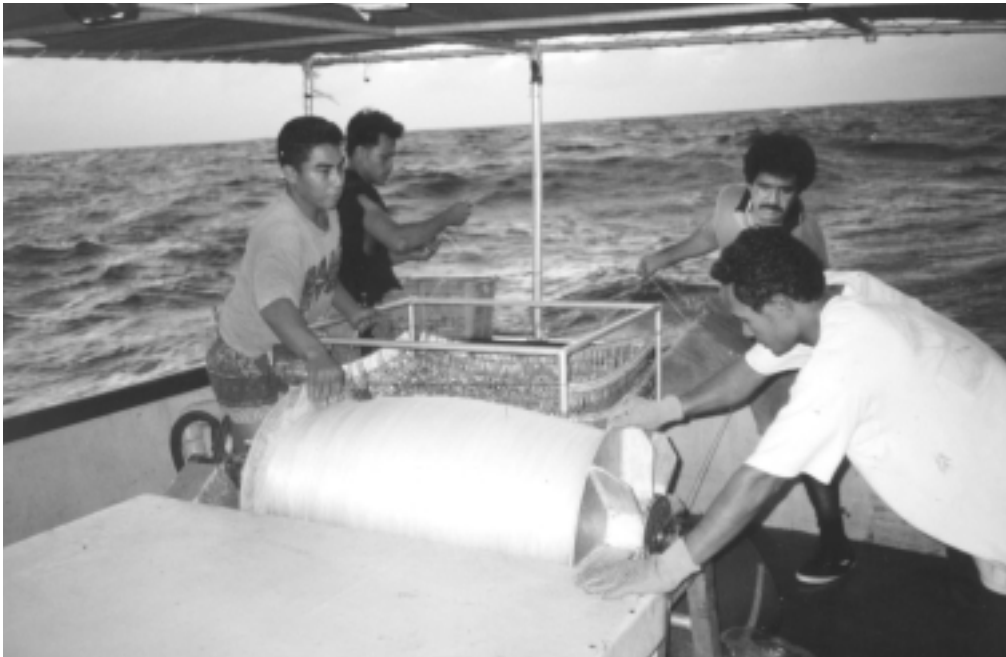
Figure 12: Slowing the reel as a butterfly knot in the mainline approaches
