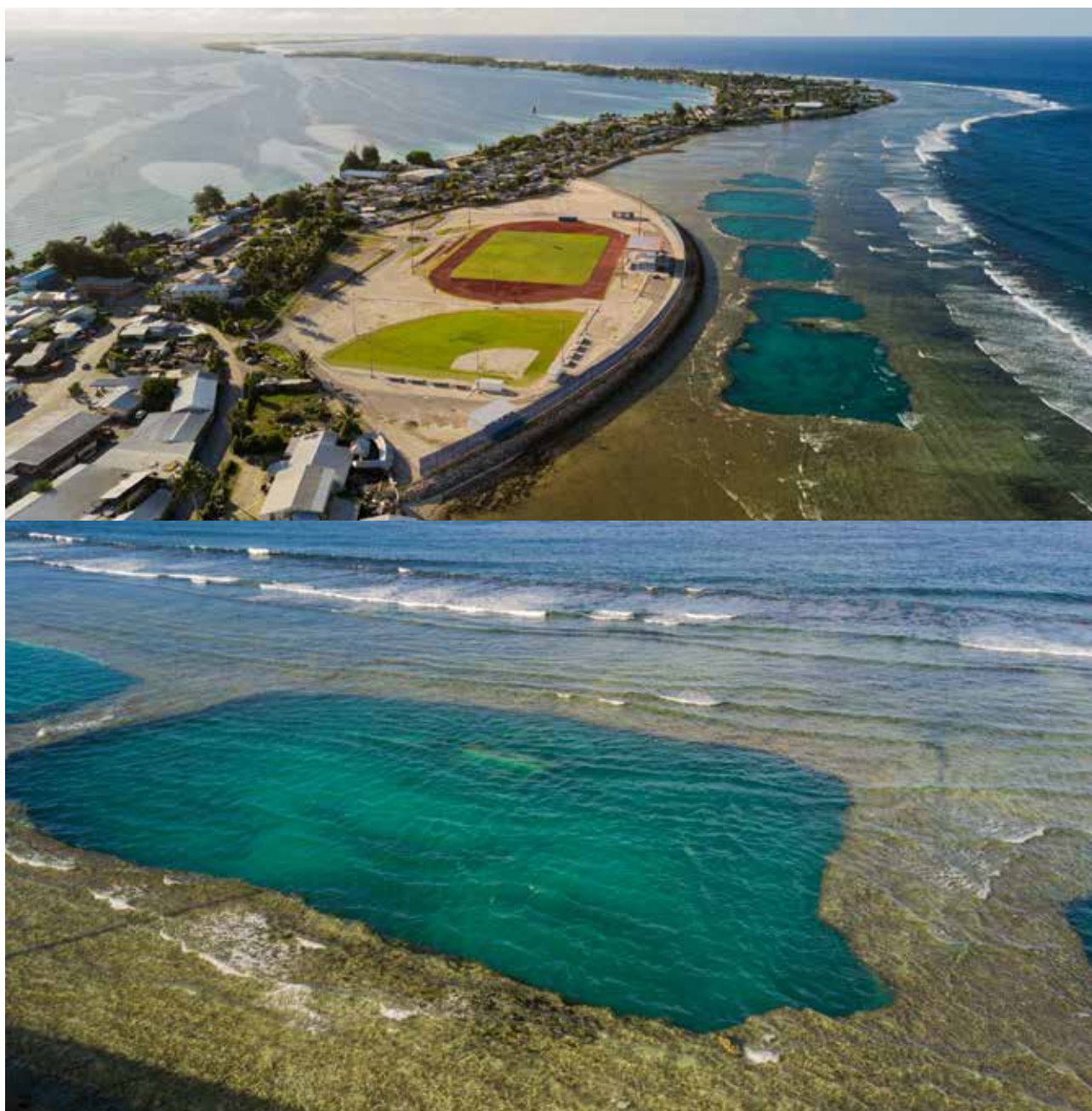
Figure 44: Reef mining pits excavated to construct the new sports stadium in Majuro.
