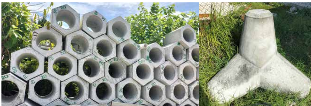
Figure 45: Examples of pre-cast concrete armour units observed in Ebeye (left) and produced by the lagoon dredging operation in Kiribati (right).
