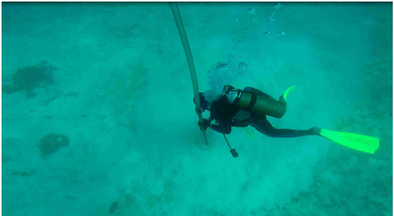
Plate 1 – Jetprobing seafloor at location JP-7.
