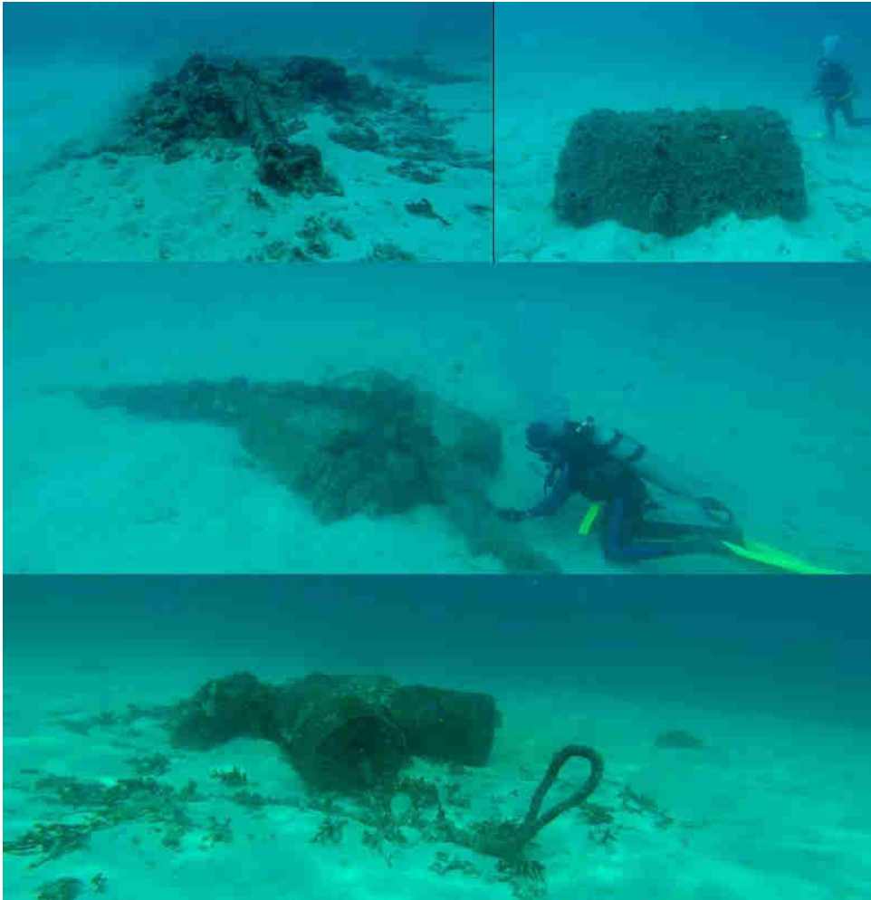
Plate 3 – Underwater pictures of targets which generated anomalies in Borrow Area 4. Top left: a large Danforth anchor on a coral patch. Top right: a large cylindrical mooring drum approximately 4x2 m. Middle: a very large mooring chain and concrete slab. Bottom: Three (3) 44-gallon drums making up a mooring. Diver provides some idea of scale.
