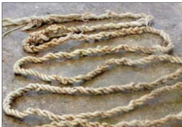
Figure 13: Hockling at around 90 m depth caused mooring line failure
