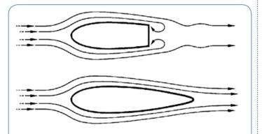
Laminar flow\* of water past a blunt-ended shape (top), which creates turbulence and drag and flow past a fusiform shape (bottom) which minimises drag.
