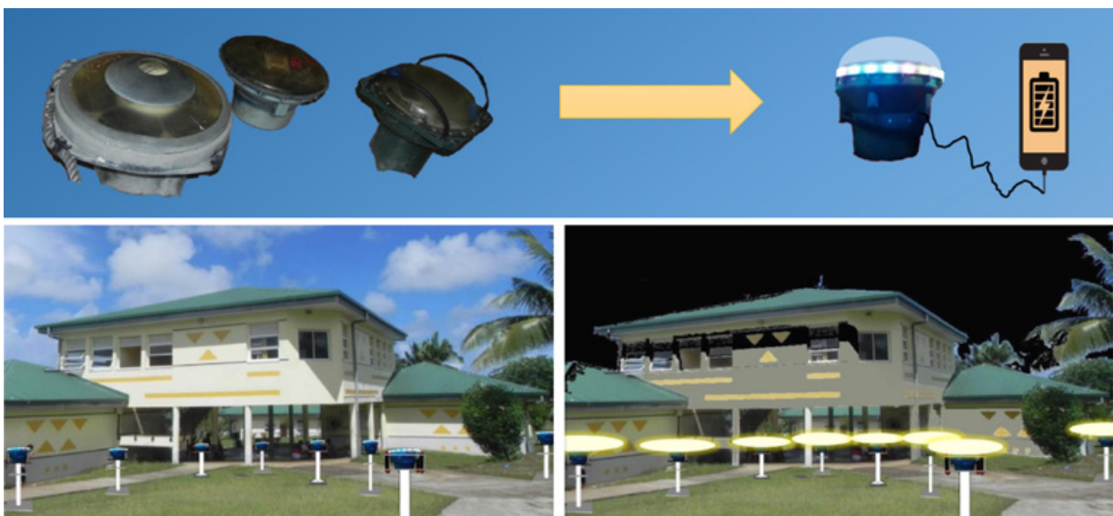
Figure 3. Mata Utu high school students re-purposed washed-up dFAD satellite buoys into autonomous outdoor solar lamps for the main entry of the school, or used as phone chargers. (images: ©Mata Utu High School)
