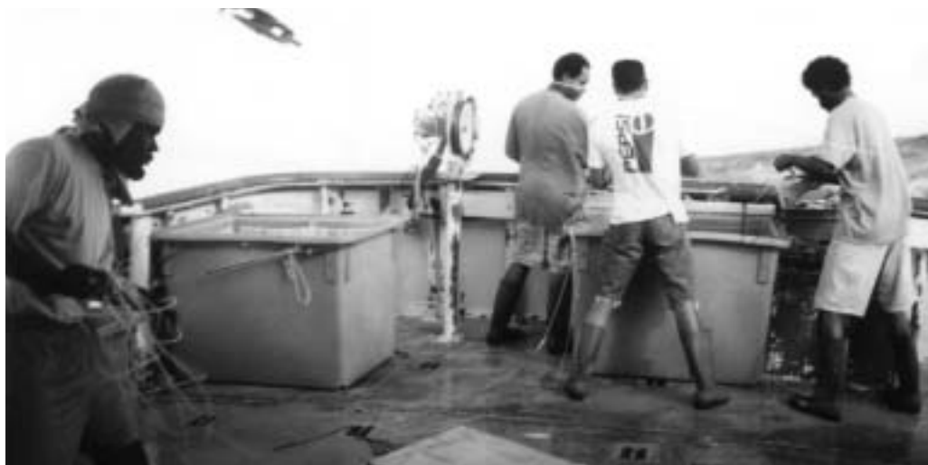
Figure 7: Mounting of line-setter on transom (starboard side of centre) on F/V Melita
