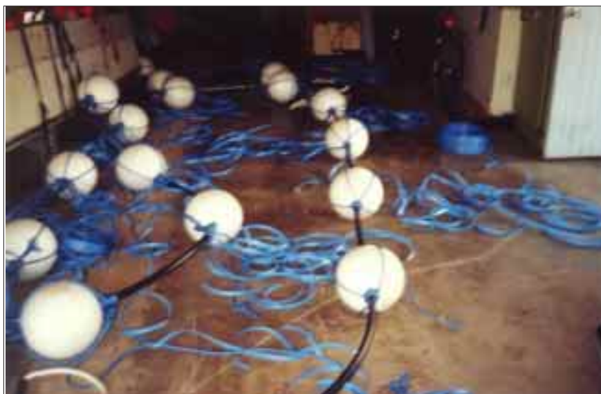
Figure 3: Aggregators to attach to the FAD buoy system [Photo: Steve Beverly]
