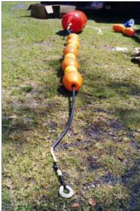
Figure 1: Shallow-water FAD buoy system [Photo: Lindsay Chapman]
