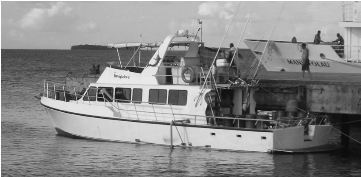
Figure 21. Photo of the survey vessel Turagalevu. The mounting pole for the 8160 Multibeam echosounder transducer can be seen over the port side.
