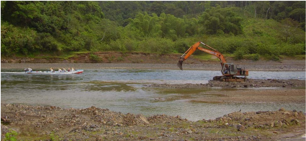
Figure 5. Gravel extraction adjacent to Nakavu Village as a tourist boat makes its way up the Navua River. Extraction of aggregates from within the river channel is increasing the sediments build up downstream from the Nakavu extraction site.
