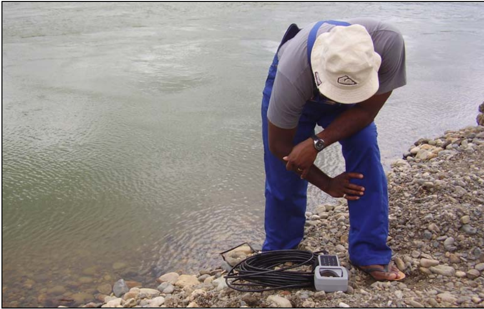
Figure 13. In-situ water quality measurements and grab samples taken for laboratory analysis in the Navua River.
