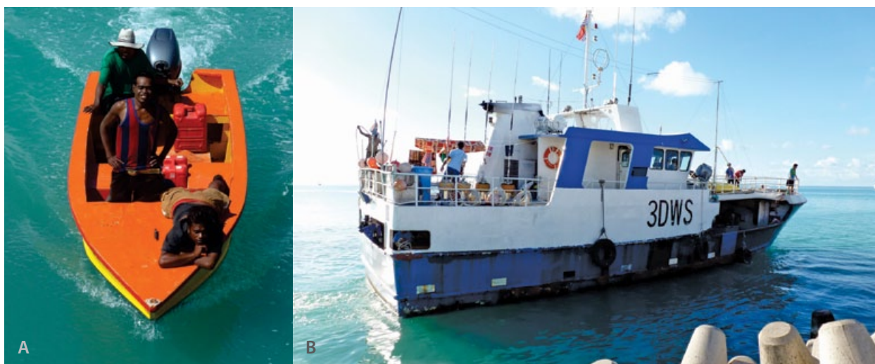
Figure 2. (A) A five-metre vessel used for skipjack trolling off Tarawa and (B) one of KFL's four tuna longliners (images: Michel Blanc).
