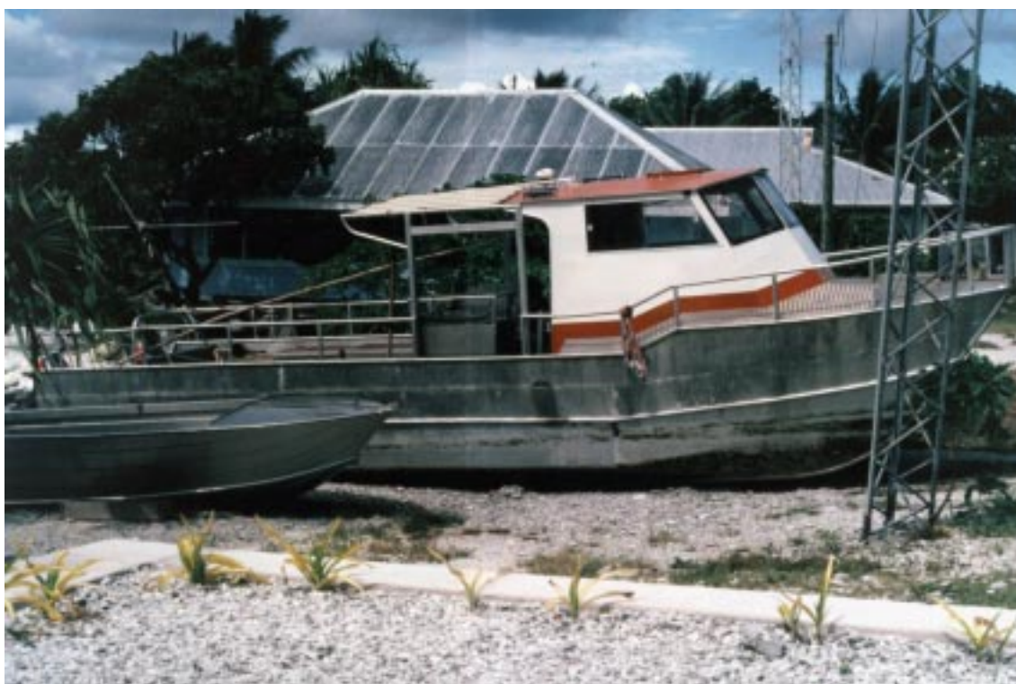
Figure 2: 12 m alia-type catamaran longliner used in Tokelau
