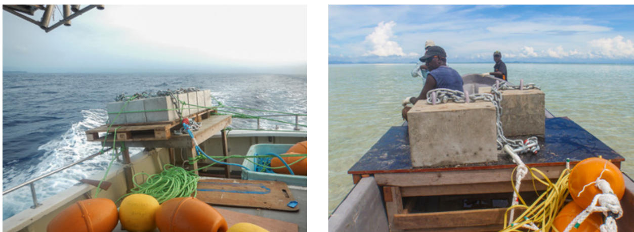
Image 9. An onboard anchor platform showing two different designs.
