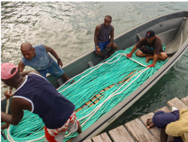
Image 8. Pre-deployment layout of ropes when using small boat deployments.
