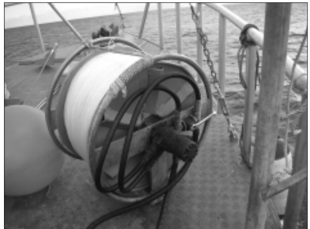
Figure 5: Clive Baxter's home-made mini longline reel.
