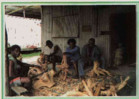
Figure 2: Chipping of sandalwood in preparation for oil extraction at a private company in Port Vila, Vanuatu.
