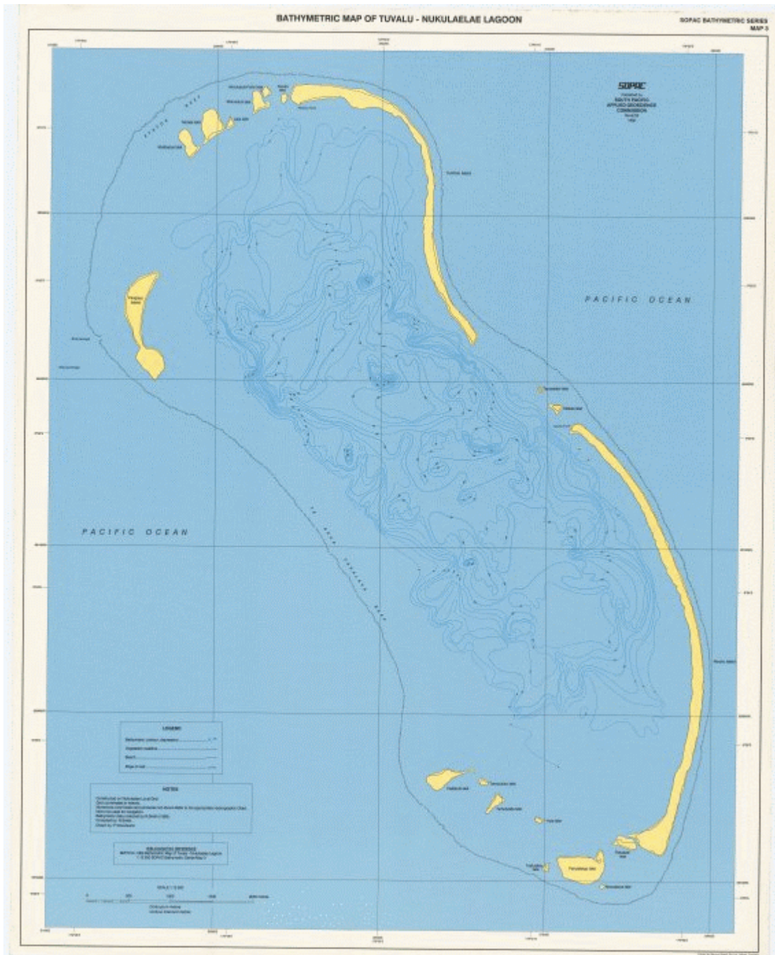
Figure 7. Bathymetry map of Nukulaelae lagoon at a scale of 1:12 500 in the original, with contours at 2-m intervals (Smith 1992a). This map is available online at the SOPAC virtual library site (see www.sopac.org ) as the Bathymetric Map Series No. 3.
