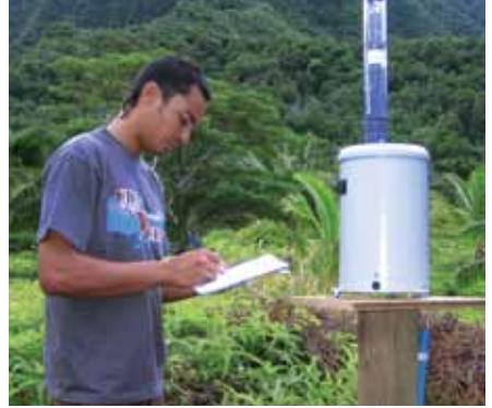
Calibration of an automatic raingauge - Rarotonga Cook Islands, 2009.
