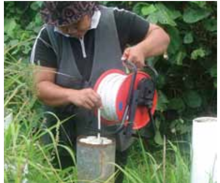
Groundwater level and quality measurement - Tongatapu, Tonga, 2008.
