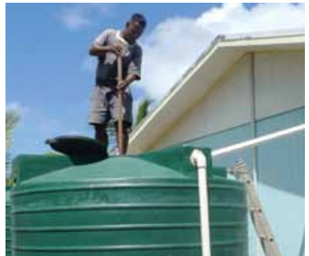
Measurement of water level in raintanks - Amatuku, Tuvalu, November 2011.
