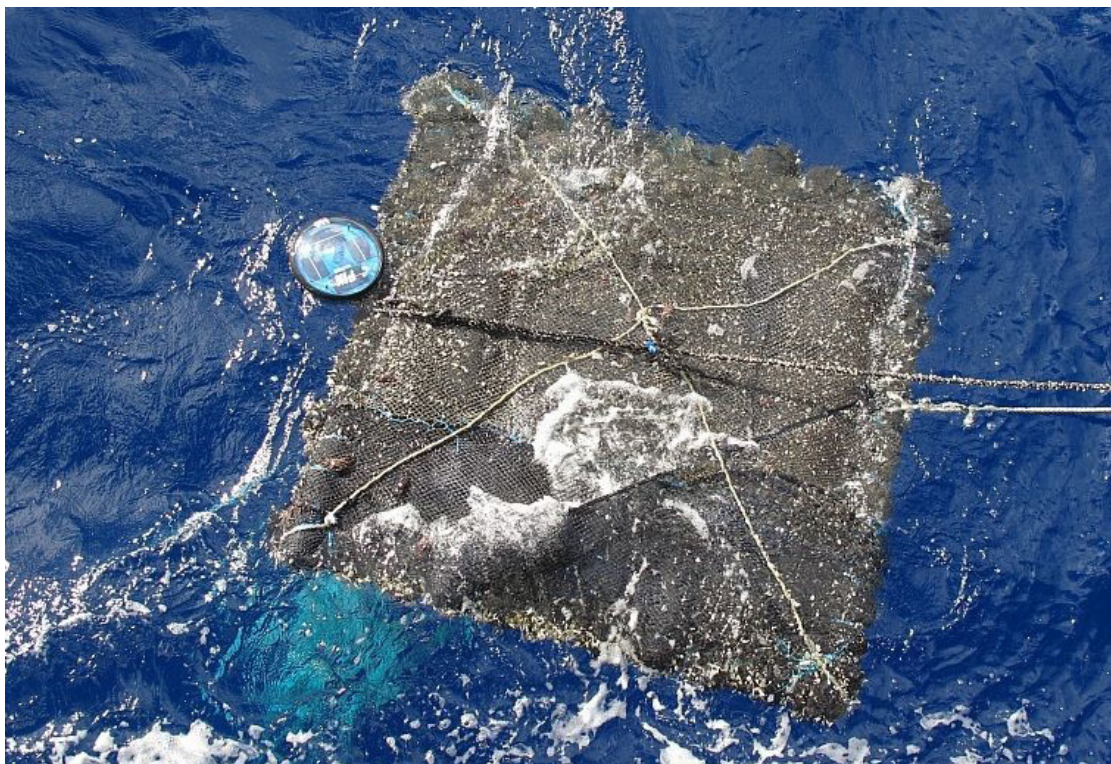
Figure 1. A drifting fish aggregating device equipped with a satellite echosounder buoy. (© SPC)
