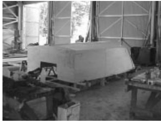
The hull with the plywood thoroughly soaked in resin
