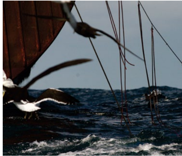
Tori (streamer) lines scare seabirds away from baited hooks as they enter the water, reducing bait loss and seabird hooking (image: Lucy Kemp, Marine Photobank)
