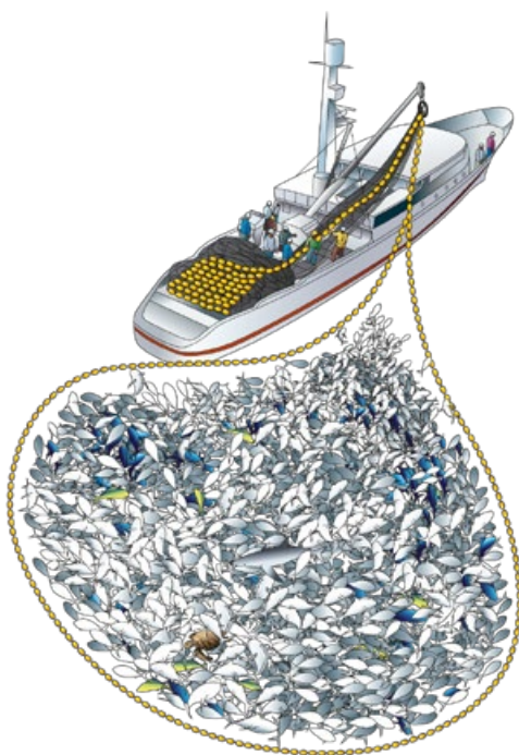
Figure 1.1 Purse seine vessel and gear
