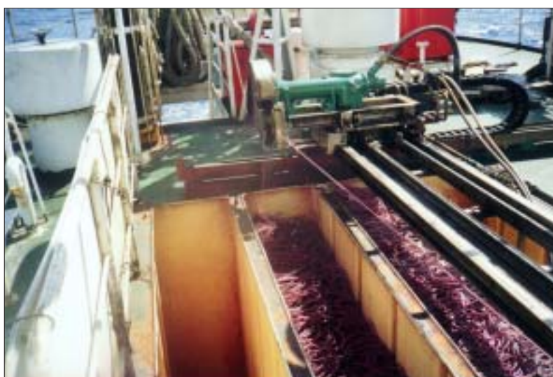
Figure 7: Mainline storage bins with rope being coiled into them
