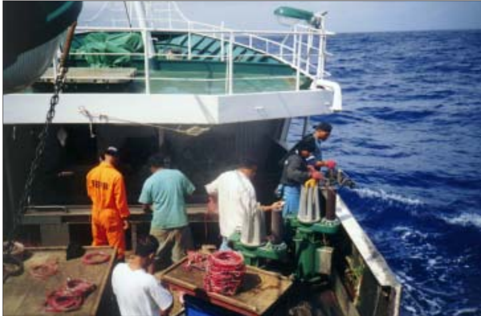
Figure 8: Coiling and stacking the branchlines from the rope gear
