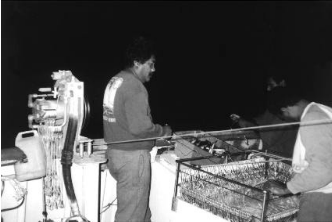
Figure 2: Setting the gear using a line thrower to increase the fishing depth of the gear
