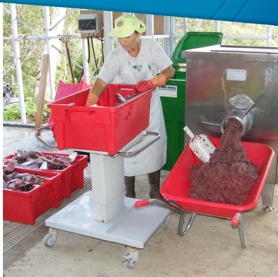
Figure 3: Small-scale operation converting tuna processing by-products into fertiliser. Photo credit: BioAgri-NC.
