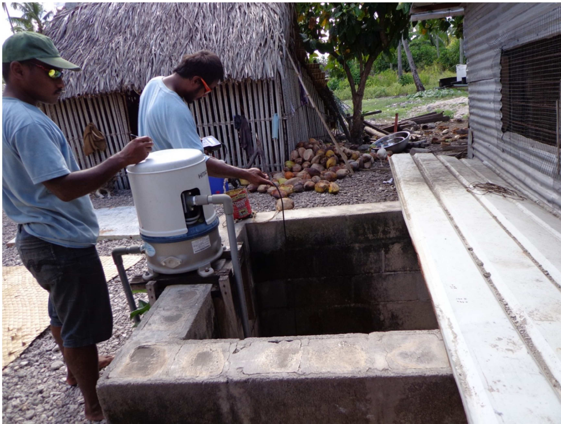
Figure A11-7. Village workers assessing water salinity level using an EC meter.
