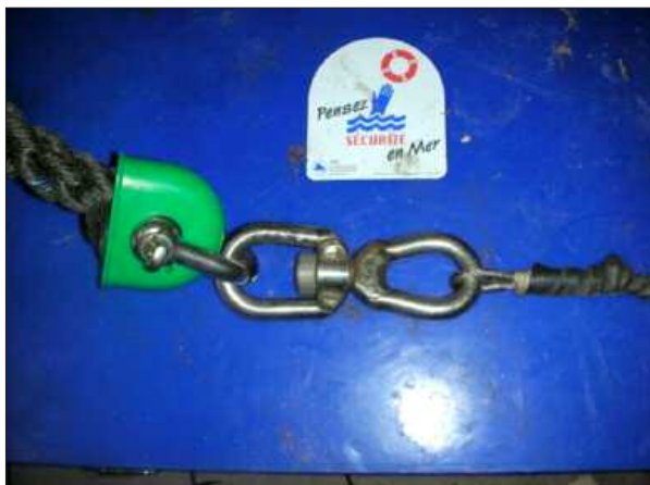
Figures 7 (left and right). Middle mooring wire; grommet spliced then secured with bulldog grips, seizing wire and bound with a rubber strap.
