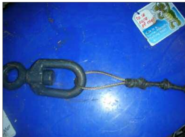
Figures 7 (left and right). Middle mooring wire; grommet spliced then secured with bulldog grips, seizing wire and bound with a rubber strap.
